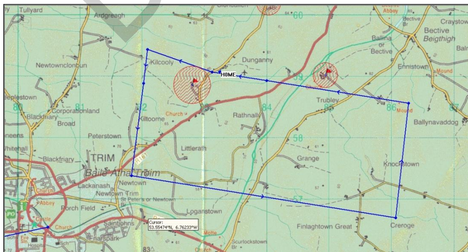
Figure 12.2: Desired Circuit Pattern for Runway 28
